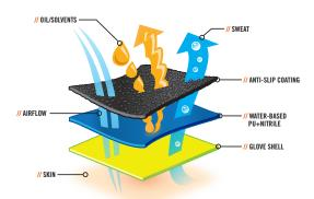
WSX<sup>™</sup> dip disperses oil/liquids from the surface while letting air flow through for breathability
