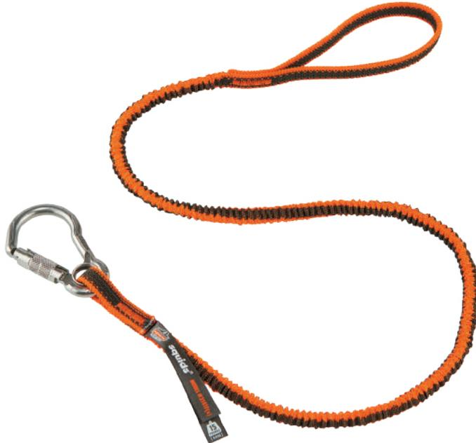
The Squids® 3101<sub>F(x)</sub> Tool Lanyard features a single stainless-steel auto-locking carabiner with captive eye on one end and a loop on the other end to tether tools up to 15lb / 6.8kg and prevent falling objects on the job. If a drop occurs, the patented design reduces force on the body or anchor point by absorbing the energy transmitted through the lanyard. This tool tether is third-party certified to 15lb / 6.8kg maximum capacity and meets the ANSI/ISEA 121-2018 standard.
